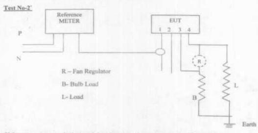
Voltage to meter terminals 1 and 2 and to the reference standard will be fed from same mains power supply.
